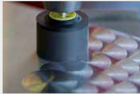
Example of a decorative finish created with an R-Flex mottling point SFM 656 on a stainless steel sheet
