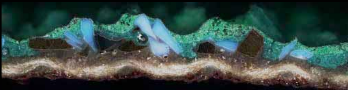
▼ Microscope image of one of the new abrasives with CEVOLUTION technology
